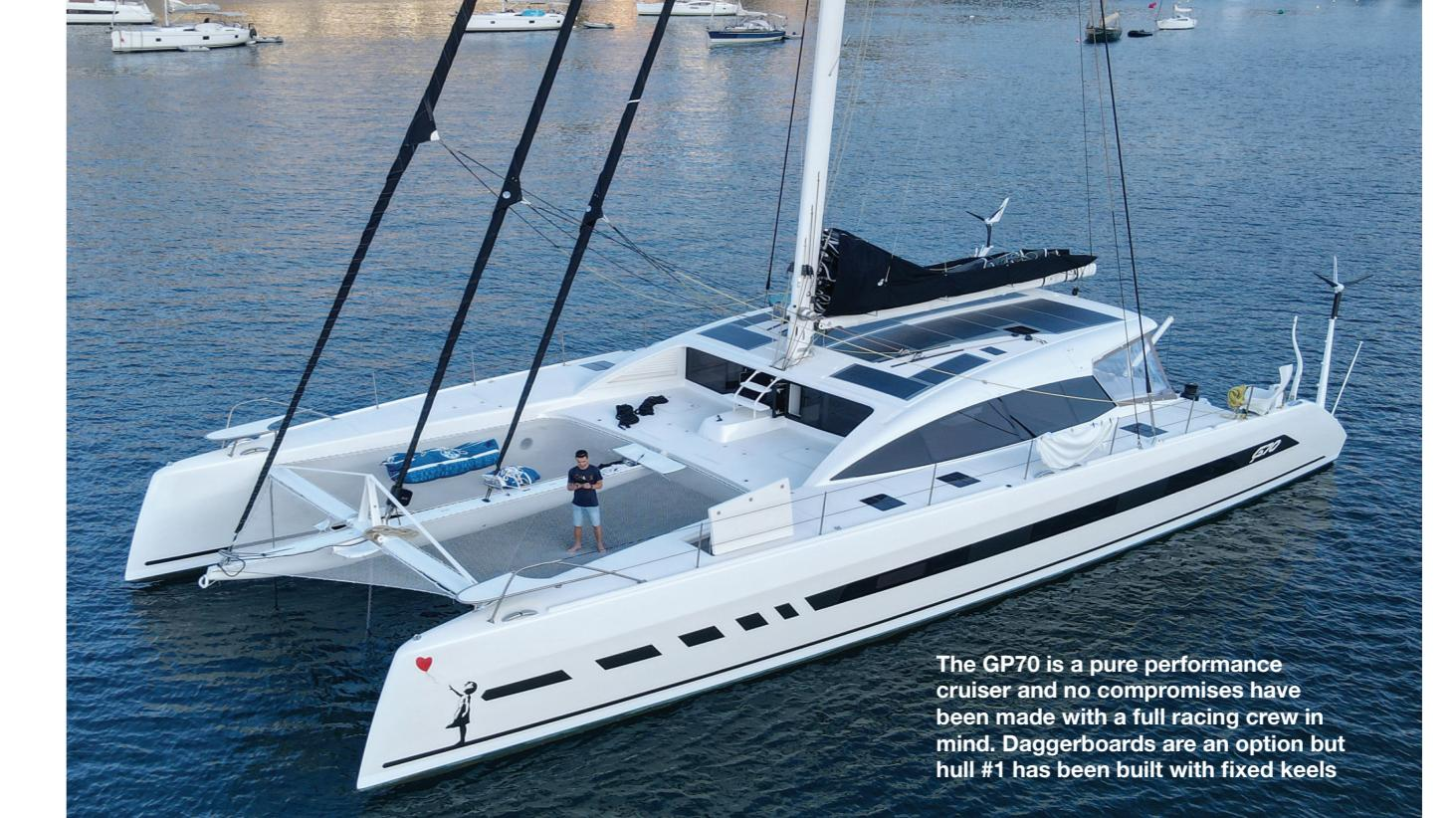
The GP70 is a pure performance cruiser and no compromises have been made with a full racing crew in mind. Daggerboards are an option but hull #1 has been built with fixed keels
