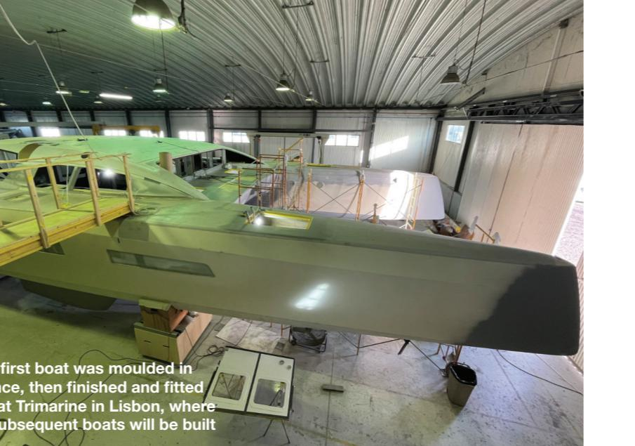
The first boat was moulded in France, then finished and fitted out at Trimarine in Lisbon, where all subsequent boats will be built
